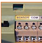
2. SENSOR OVERRIDE "ON/OFF" SWITCH 24 VAC INPUT EXTERNAL
